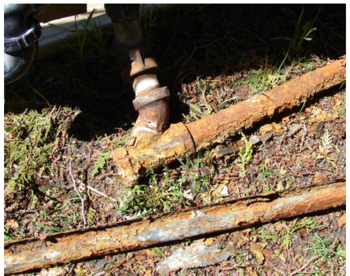
This is the corroded pipe from under the bar sink, with over half of the pipe missing.
